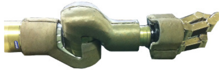
Figure 6: The capacitive tactile technology developed during ROBOSKIN project, integrated on the Schunk arm
