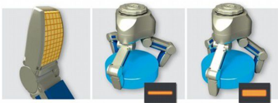
Figure 11: SCHUNK SDH-2 with tactile sensors measure forces and torques.
